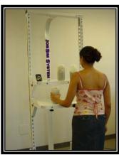
One shelf is placed at the subject's waist level and a second shelf is placed 25 cm above it. The three 1-kg containers are placed 10 cm apart, in line with the screws on the upper shelf, on the lower shelf.
