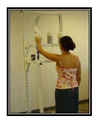
One shelf is placed at the subject's eye level and a second shelf is placed 25 cm below it. The three 1-kg containers are placed 10 cm apart, in line with the screws on the upper shelf, on the lower shelf.
