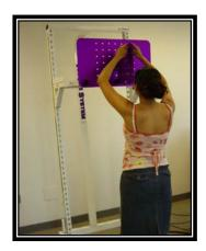
A shelf is placed at the subject's eye level with an attachable plate, perpendicular to the shelf, projecting out toward the subject.
