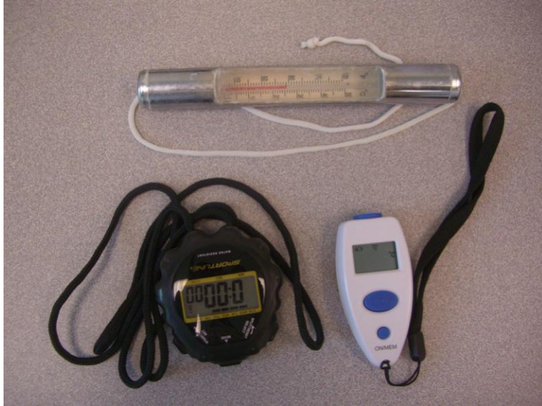
Figure 2: Instruments of CST: Top- Pool thermometer is for cold water temperature measure inside the insulated container ; Bottom Right-Temperature recording Infrared Skin thermometer is used to measure temperature of the target digit ; Bottom Left- Stop watch for time monitoring
